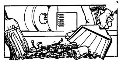
Keep electrical equipment, machinery and work areas clean to prevent electric fire hazards.
